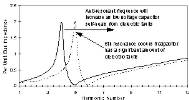
Fig. 7 - Shift in Tuning Frequency Due to Loss of Capacitance in Low Voltage Capacitors
