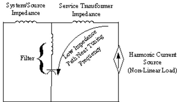
Fig. 5 - Equivalent Circuit of System Shown in Fig. 4
