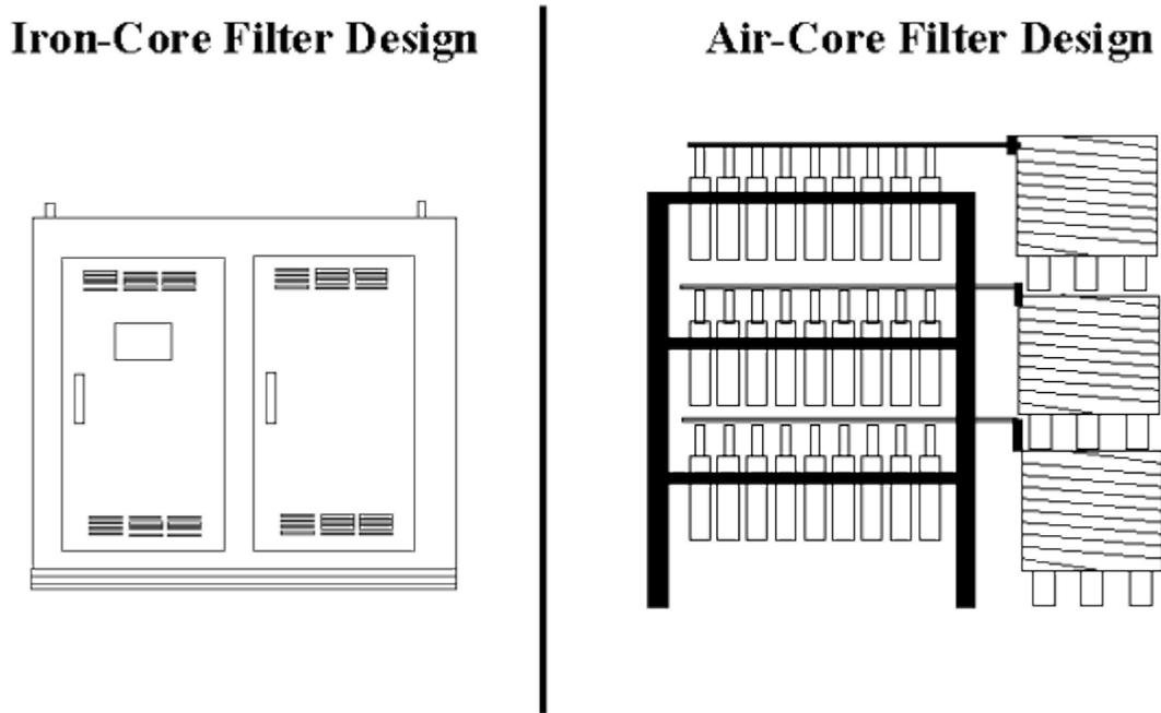
Figure 2 - Typical Iron-Core and Air-Core Filter Designs
