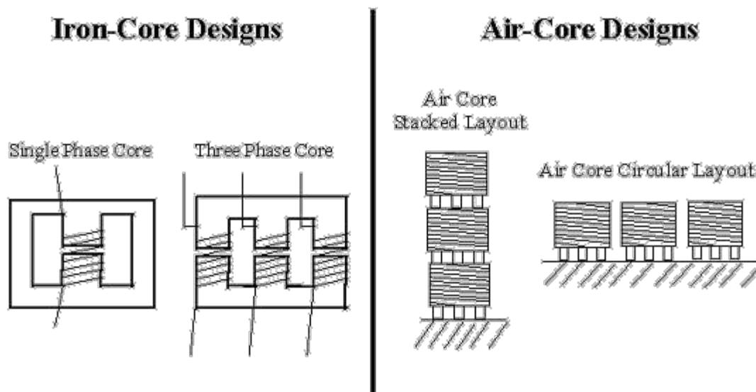
Figure 1 - Typical iron-core and air-core reactor designs
