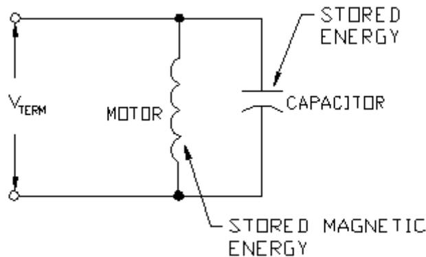
Figure 2 - Simplified Circuit Diagram for Motor Controller and Power Factor Correction Capacitors (Diagram Shown For Motor Controller in Open Position)
