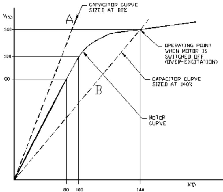
Figure 3 - Typical Motor Saturation Curve and Capacitor Characteristic Curves at a given frequency
