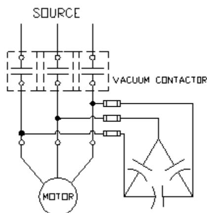
Figure 1 - Typical Power Factor Correction Capacitor Application On Induction Motor
