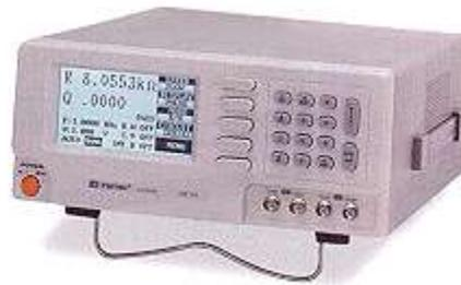
*Figure 7 - A High Precision LCR Meter With an Accuracy On The Order of 0.05% in the Picofarad Range is Required to Ensure Equal Capacitance Across the Vacuum Bottles*
