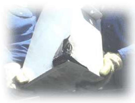
*Figure 2 - Restrike Caused 5 Capacitors to Rupture Like the Opening of a Sardine Can as Shown Above*
