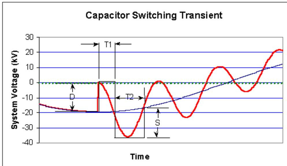
Figure 4 – Height, Depth, and Time of Voltage Dip and Spike Shown On Transient Waveform
