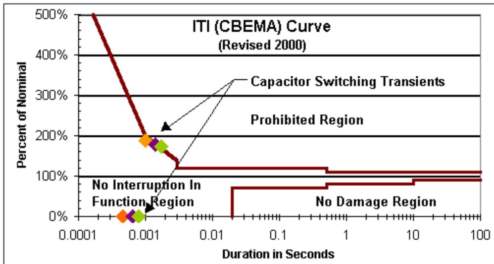
Figure 5 – ITI (CBEMA) Curve Showing Voltage Dip and Spikes Caused By Various Size Capacitor Banks
