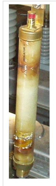
Figure 3 – Picture of a Failed Fuse Due to Over-Heating
