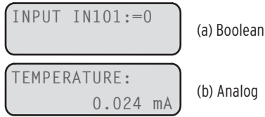
Figure 4.74 Front-Panel Display for an Entry in (a) Boolean Name and Alias Strings and (b) Analog Name and User Text and Formatting Strings
