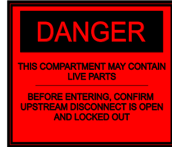
Above tag to be placed on air-disconnect internal barrier door.
