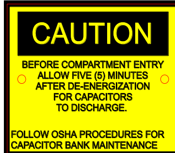
Above tag to be placed on all capacitor bank access doors.
