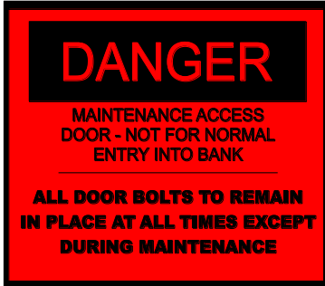
Above tag to be placed on all bolted access doors that are not equipped with key interlocks.
