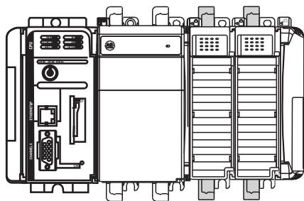
In a 1769-L3x controller system, the 1769 I/O modules can be placed to the left and the right of the power supply. As many as eight modules can be placed on each side of the power supply.
