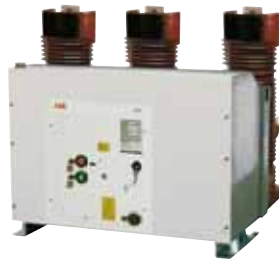
Fixed HD4 36 kV circuit-breaker with 350 mm pole centre distance: I r = 630-1250-1600 A; I sc = 16-20 kA.
