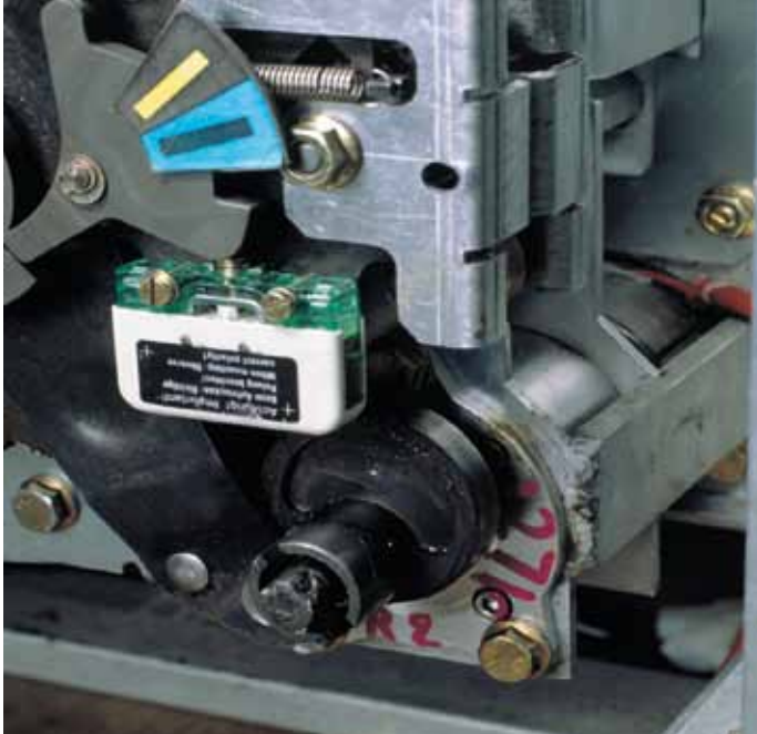
Spring charging geared motor.
